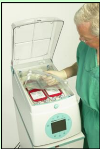
fig. 1: Barkey plasmatherm with 4 blood bags and opened cover.
